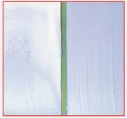
coatings. Results show that after five days in a caustic solution, the other waterproofing coatings (left) displays severe degradation, while Lanco® **Dry-Coat™** remains relatively unaffected.
